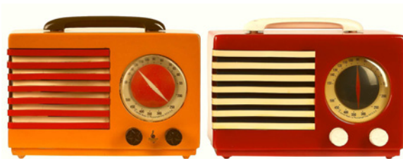
Figure 28 Norman Bell Geddes, [k] 1940: Radio Patriot 400, cast phenolic resin cabinet, Emerson Radio & Phonograph Corp., USA. [67]
