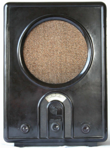
Figure 24 Walter Maria Kersting, [9] 1933: Radio Volksempfänger VE 301 W, pressed phenolic resin radio cabinet. [47]
