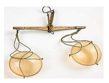
Figure 2 Pharmaceutical hand scale with cellulose nitrate pans. Early 20th century. [6]
